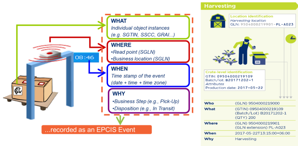
Figure 32: How EPCIS used in supply chain
